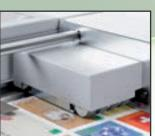
The pile feeder is using a vacuum belt technology and air knife control for a perfect sheet separation. It handles paper sizes from 105 x 148 mm to 375 x 1'050 mm.
