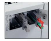
The creasing and perforating tools are automatically letected and the relevant pressure is automatically set. No manual adjustments are needed.
