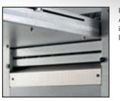
An online perforating device is available for the lower exit level as an option.
